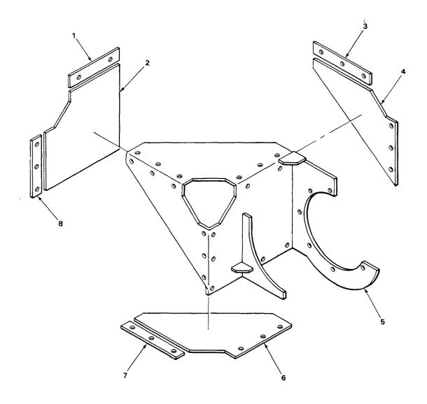
Figure 4. Bracket Assembly, Cradle.
